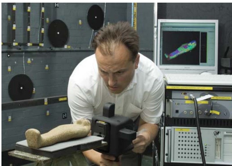
Professor Stuart Robson colour laser scanning an object from the Petrie Museum.
